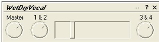
Figure 4. Audiomulch Crossfader mapped to the right slide sensor controlling the amount of signal sent to processors.
