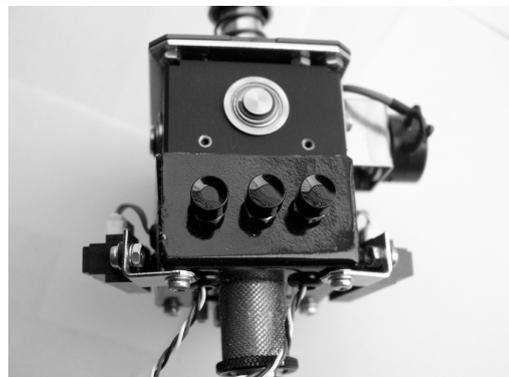
Figure 16. Switches on joystick casement.
