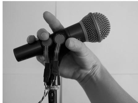
Figure 9. Grip pressure sensors.
