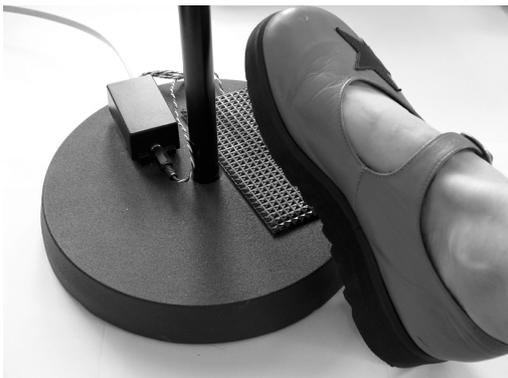
Figure 7. Foot pressure controller.
